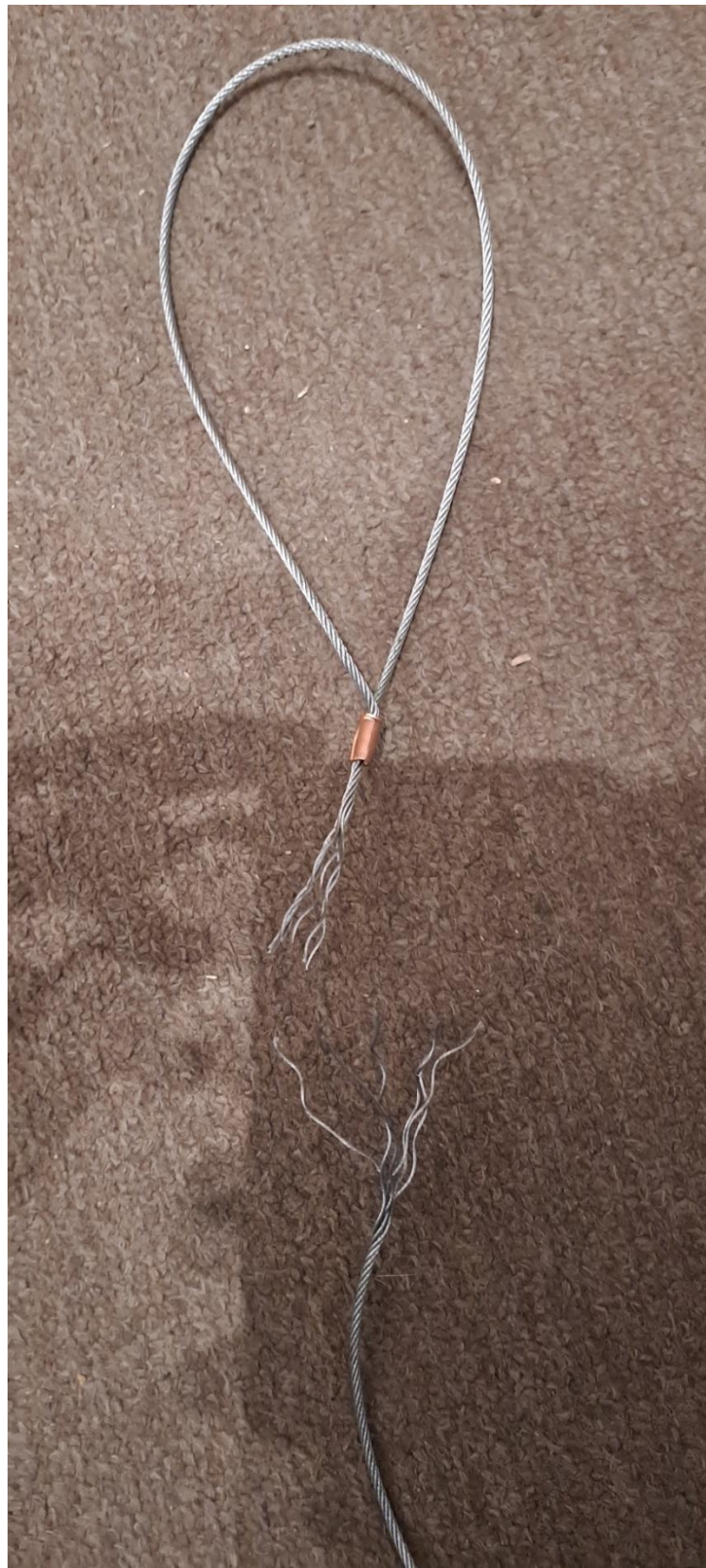
Fig. 12 Sample of steel cable with Nicopress sleeve after the test
