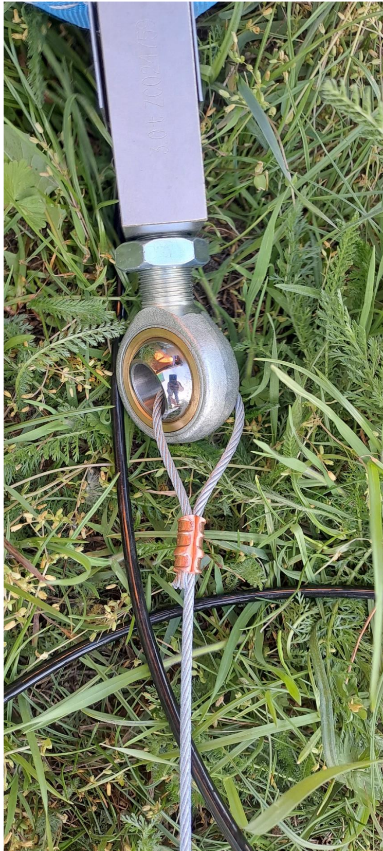
Fig. 10 Tested part of steel cable with Nicopress sleeve, from the tension sensor site
