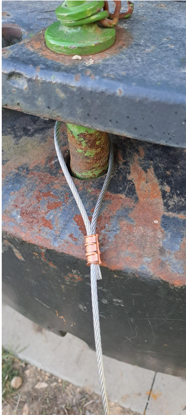
Fig. 11 Tested part of steel cable with Nicopress sleeve, from the vehicle site
