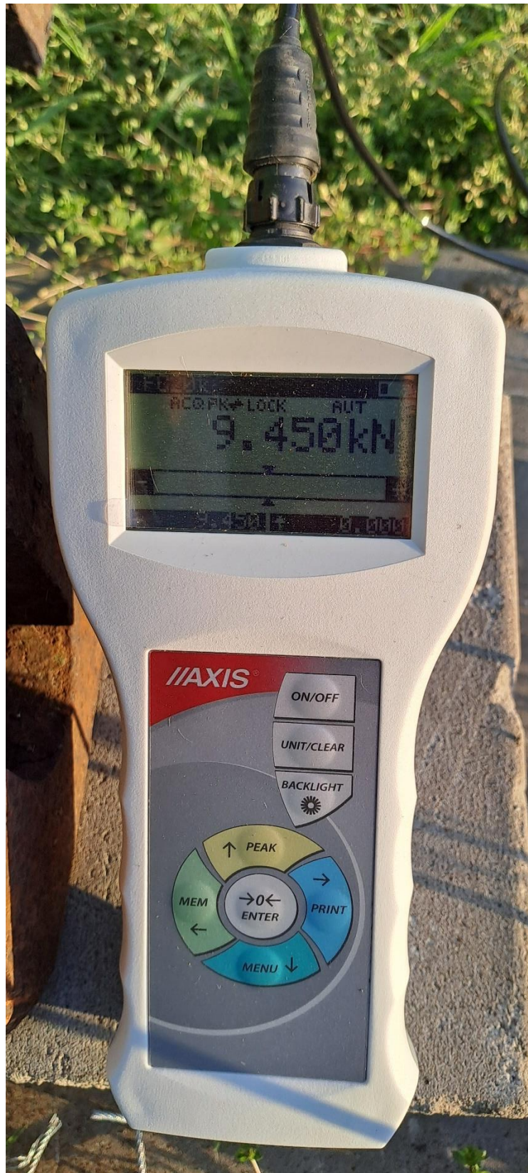
Fig. 15 Value of actual destructive strength for 3,2 mm steel cable
