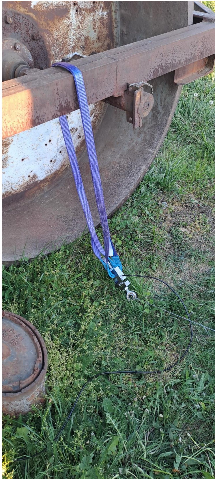
Fig. 9 Tested set – belt, tension sensor and steel cable with Nicopress sleeve
