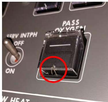
Figure 1 – Example of Breakaway Wire on PASS OXYGEN Switch Guard
